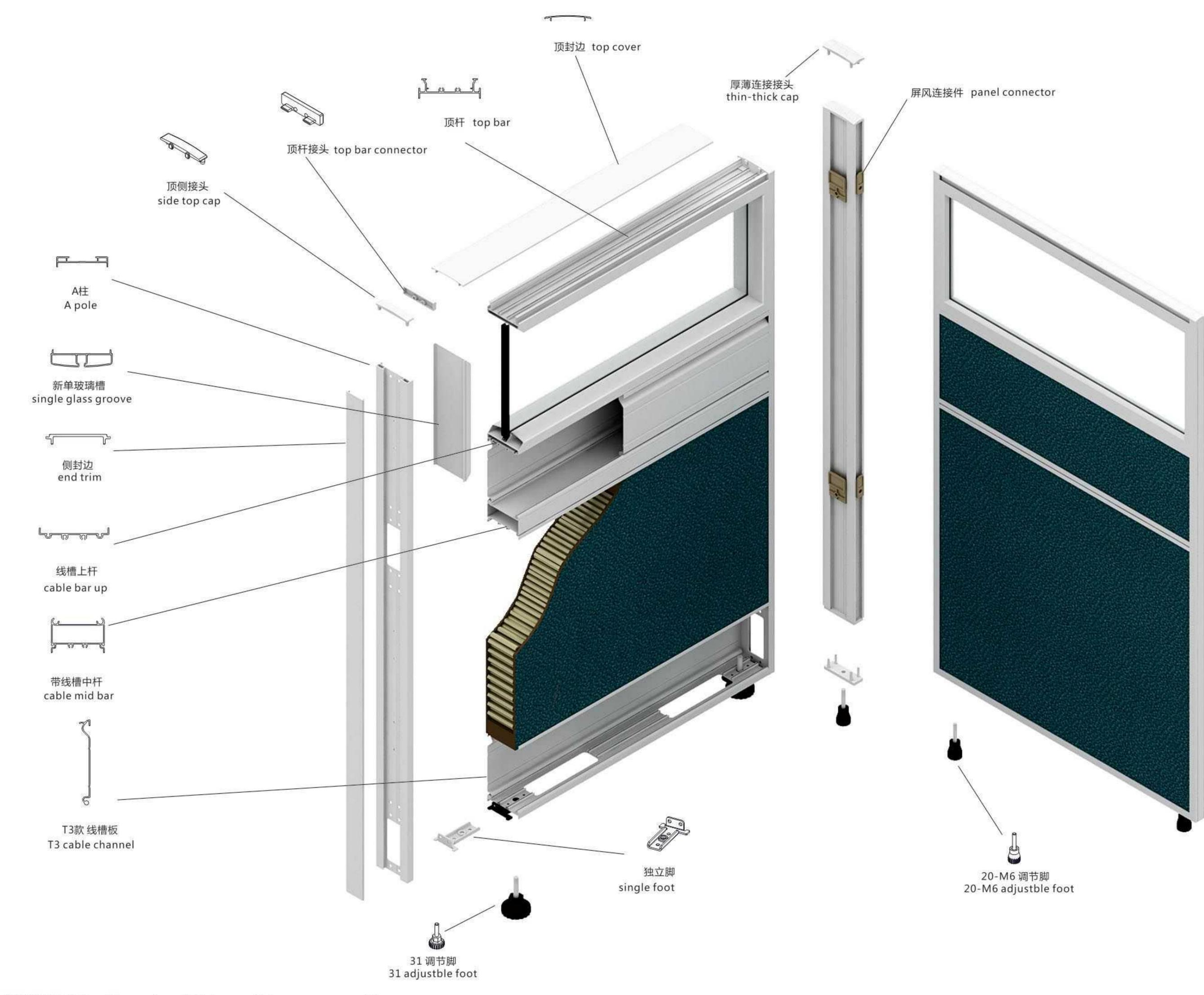
C系列厚薄连接柱 C series Thin-wide connection
